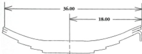
Trailer Spring, Six Leaf, Low Arch 24,000 lb. capacity. Replaces 751-04
